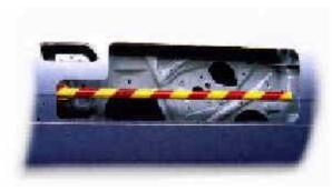
Looking at the picture aboveyou should say that Citroën has designed the Xantia carefully, together with the high tensile steel bars in all four doors. This together with the
